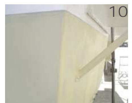
Repair revealed after soda blasting
